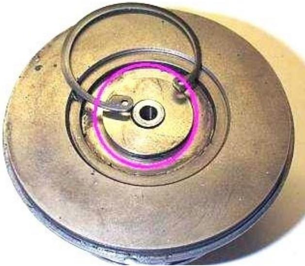
The circlip removed. Note the circled area on the end cap - there is a raised lip here.
