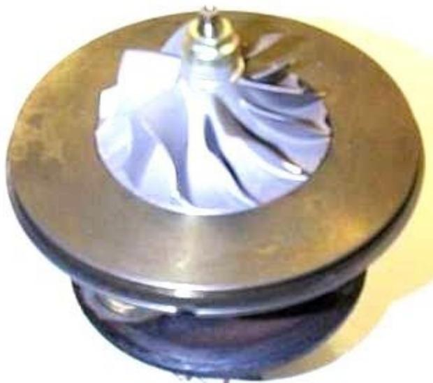
Turn the center section over and slip the compressor wheel onto the shaft. ***If you scribed marks on the shaft, wheel, and nut, now is the time to line them up.*** Then torque the nut to 70-78 in-lb. (***not*** ft-lb.!!!). It might be best to use some blue threadlocker on this nut, even though most I've seen are self-locking.
