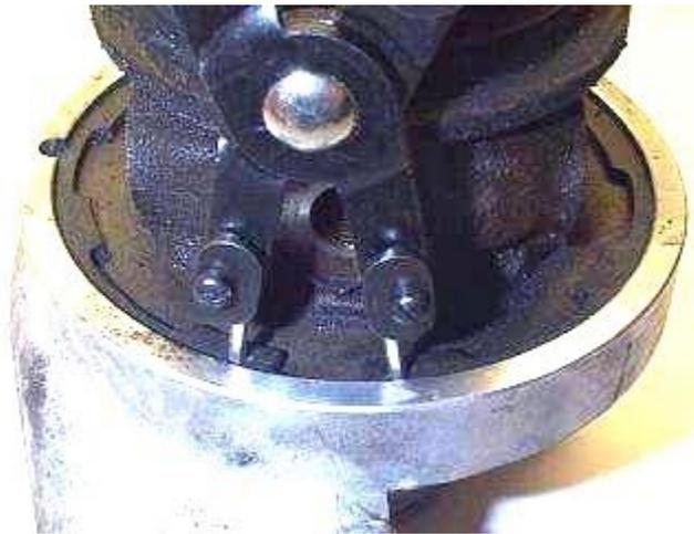
Circlip pliers in the ends of the circlip. I got the "deluxe" circlip pliers from Sears, they can be converted from inside to outside pliers instantly, and have several tips. I install the tips backwards in the pliers for this large circlip, because all the tips taper down to small ends that would break off when trying to move a circlip this large.
