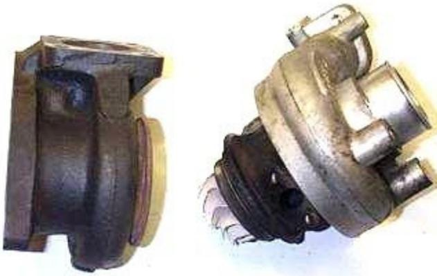
Pulling the turbine housing from the center section. You may need to hold the compressor side and tap the turbine housing with a hammer to knock it loose. If so, hold the turbo barely above a pillow or something to catch it, hold the turbo with the turbine housing straight down, and strike at it parallel to the turbo centerline, so when it comes off, it comes straight off, and does not hit the turbine blade.
