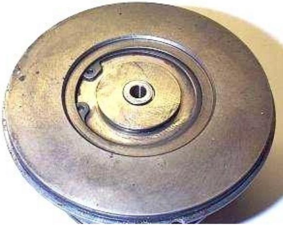
Here's a compressor side view of the center section with the turbine shaft removed. The circlip holds a center cap in place.
