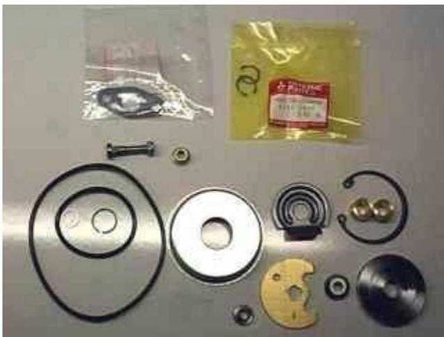
Here's a 16G rebuild kit. *Note* that it is different than a 14B rebuild kit. The center cap has a different profile to match the backside of the 16G wheel.
