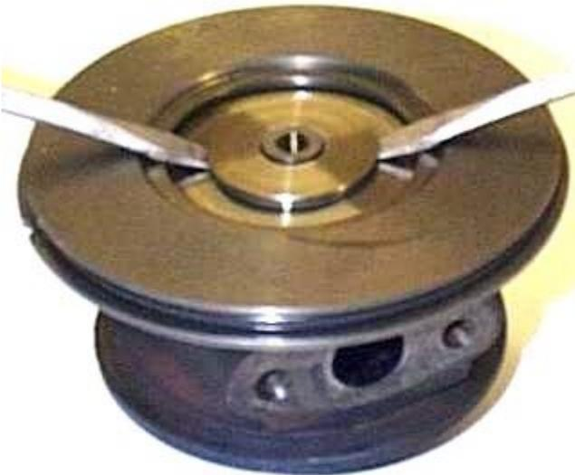
Place 2 flat blade screwdrivers 180 degrees apart under this lip, and carefully pry the end cap up and out of the center section. You might need to move the screwdrivers around the lip and gradually pry it out, depending on how tight it is in there.
