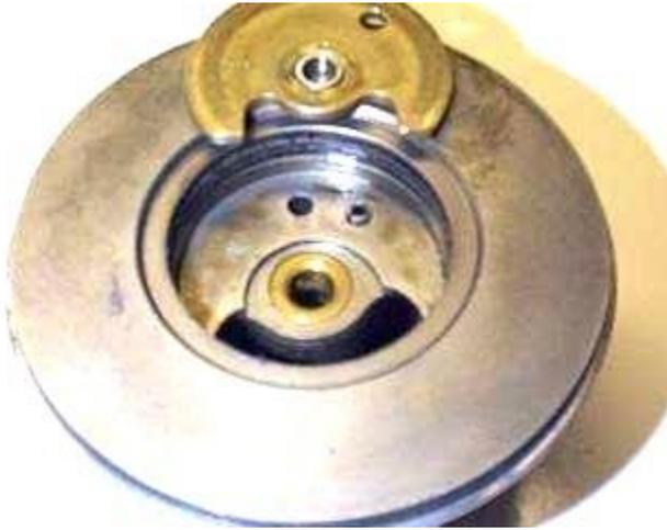
The brass thrust bearing sitting on the center section, oriented as it is in the center section. Note the steel bushing in the center of the thrust bearing. Note the hole in the thrust bearing that fits over the rollpin in the center section.
