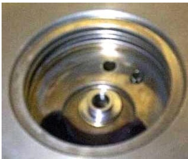
Place the thrust bearings' steel bushing onto the center bearing.
