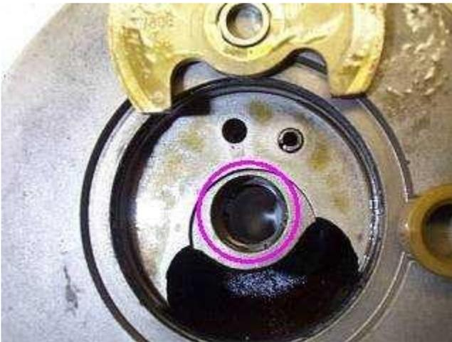
Circled is a tiny circlip inside the center section. There is one on each side; they keep the center bushings from slipping into the center. I removed them using two pins to contract them, then pushed them out of their groove, then pulled them out with needle nose.
