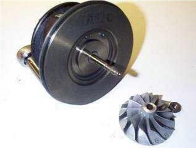
The compressor wheel off of the center section. I didn't scribe the wheel and shaft because I had combined parts from several turbos, and sent the turbo off to be balanced after the rebuild.
