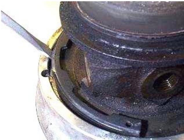
This is after the clip is loose, but while you have the pliers contracting the circlip, stick a screwdriver under the circlip, and pry it up and out of its groove, then work it off of the turbo. **BE VERY CAREFUL**, this clip is large and has a lot of force, it is hard to remove, and if you slip, it can hurt.
