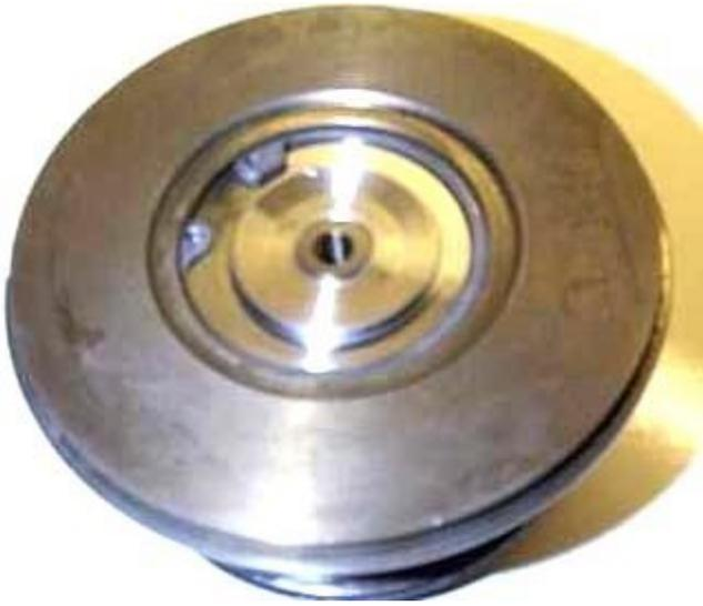
Press the center cap into place and reinstall the circlip.
