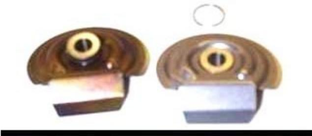
The old 14B spring plate and bushing on the left, 16G on the right. The top pic shows the spring plate, bushing, and sealing ring. The second pic shows the bushing in place, with the sealing ring above it. Carefully slip the sealing ring over the top of the bushing. It will be a loose fit. The bottom pic shows the spring plate assembly ready to go into the center cap.
