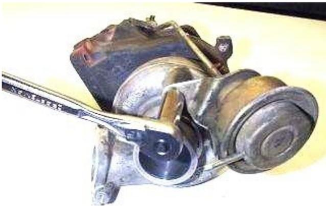
Removing the wastegate actuator (12mm).
