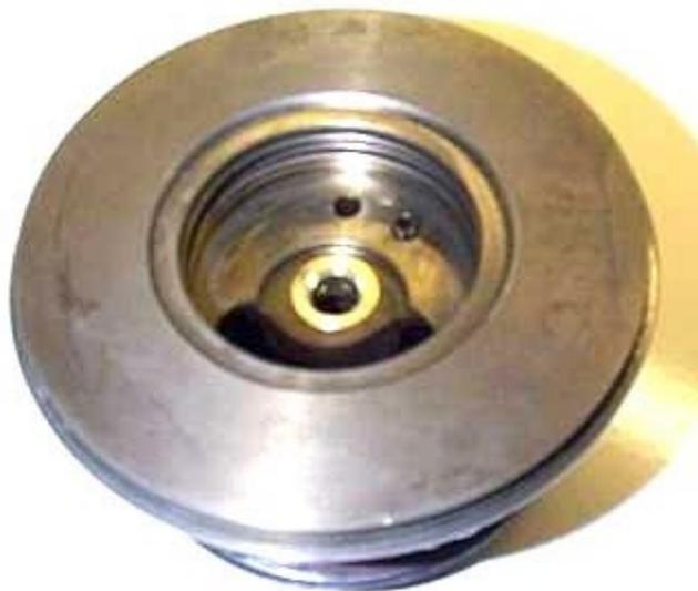
After installing the small center bearing circlips (not shown, as I did not install them, due to the pending Forced Performance work), place the compressor side brass bearing into the center section.
