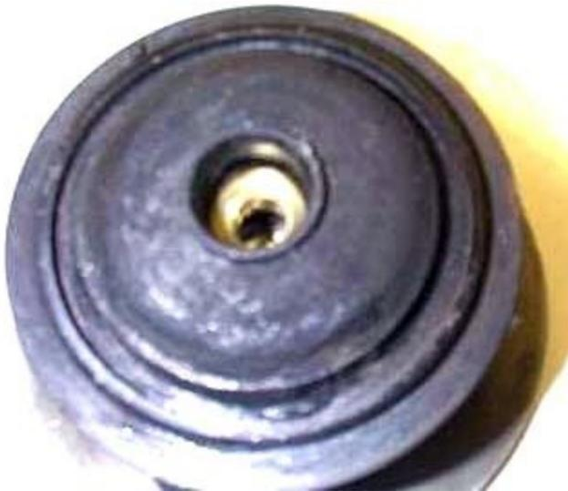
Install the turbine side center bearing into place. Again, note that I did not fully clean the center section, as I sent the turbo off to Forced Performance for a thorough cleaning, machining, reassembly, and balancing.
