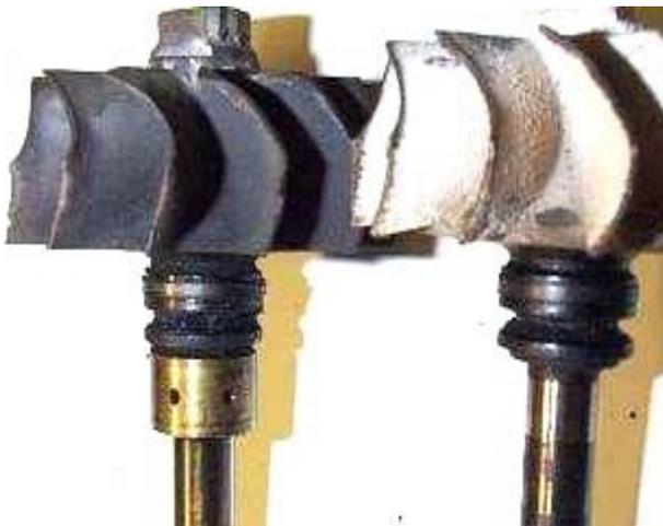
Left side, *bad*, right side, *good*. The left turbine wheel got torn up when something went through the turbo. Note the valley in the shaft that is pretty grainy on the left side - this is after cleaning it with a screwdriver. The right side shaft was almost as bad, I used a screwdriver and followed up carefully and lightly with a razor scraper, it is almost totally clean. Note the left shaft still has the bushing on it; I have removed the one on the right shaft. It just slides on.
