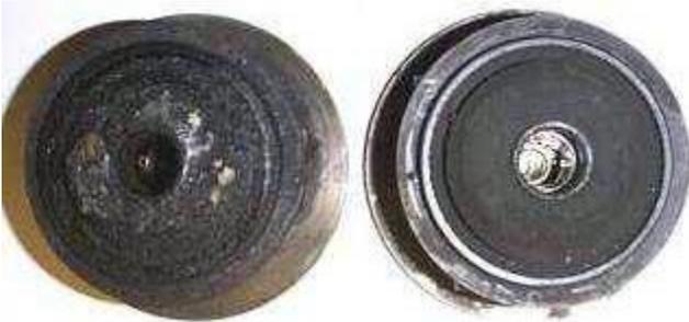
The center sections of two 14Bs, after the sheet metal guard is removed. Left side, *bad*, right side, *good*. The left side shows *severe* coking. The shaft had *totally* locked up, but after cleaning all the coking off, it spun well again.
