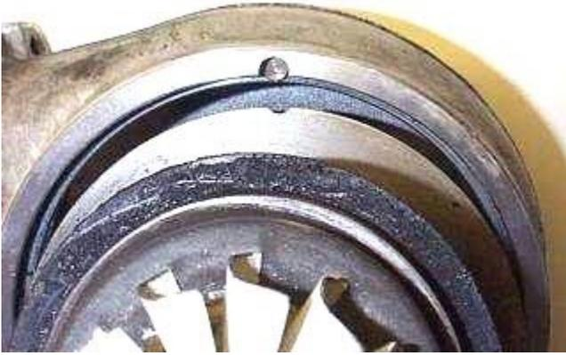
Here's the center section out of the compressor housing, a better view of the locating pin.
