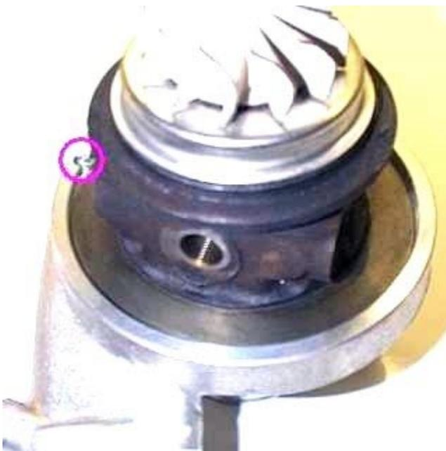
Place the center section into the compressor housing, making sure to line up the locating dowel in the housing with the notch in the center section.
