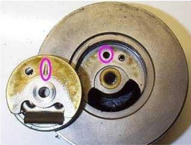
The center cap and thrust bearing turned over. Note the oil feed journal in the thrust bearing, fed by the circled hole in the center section.
