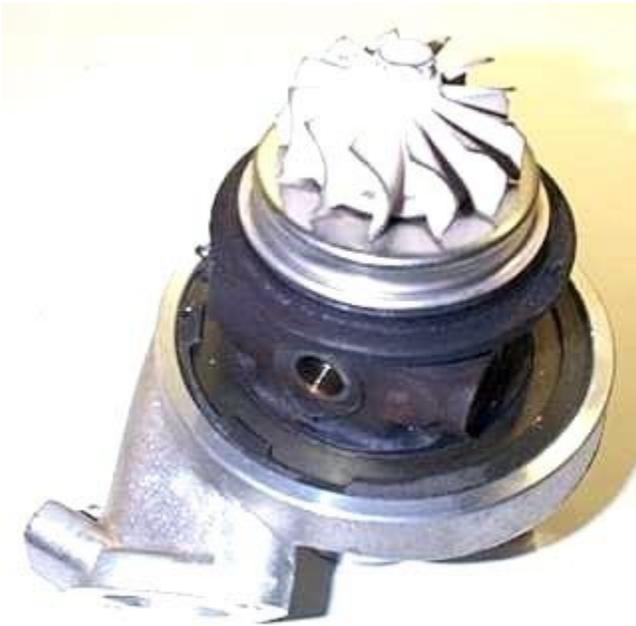
Install the compressor housing circlip.
