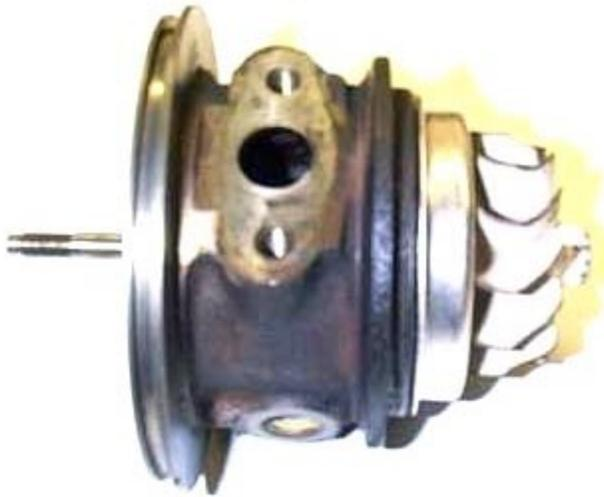
Carefully press the turbine shaft into the center section. You will feel it "click" into place when the turbine shaft sealing ring compresses.
