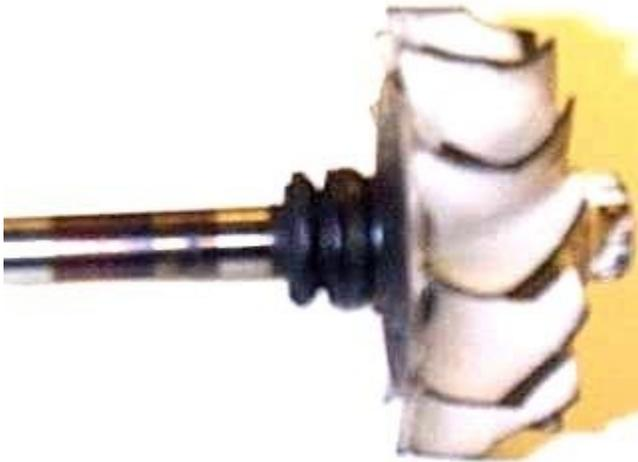
Here is the old turbine shaft and wheel, with the old sealing ring in place.
