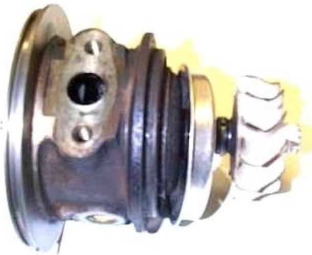
Place the new heat shield on the center section and carefully slide the turbine shaft through the center bearings.
