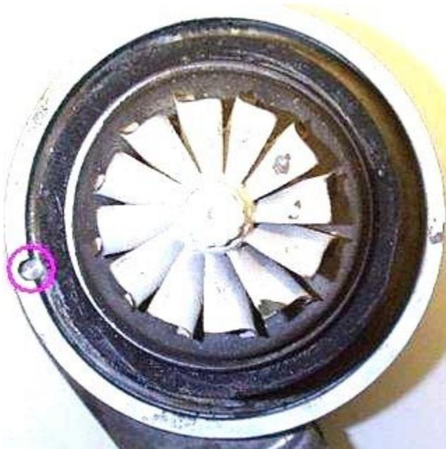
Circlip gone. The circled area is the locating pin.
