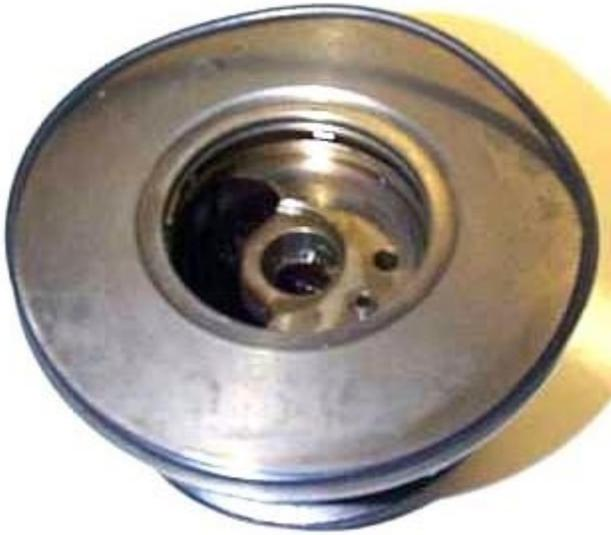
Install the new compressor housing and center cap O-rings (ignore the fact that my center section is not clean, I did not install the O-rings, I sent it to Forced Performance without some of the parts installed to make disassembly for a *thorough* cleaning easier).
