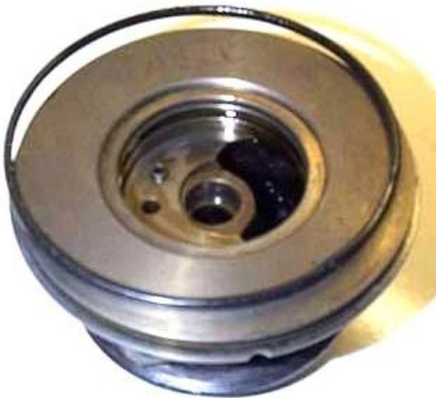
Remove the compressor housing O-ring. Mine broke in several places while removing it, as it was dried out.
