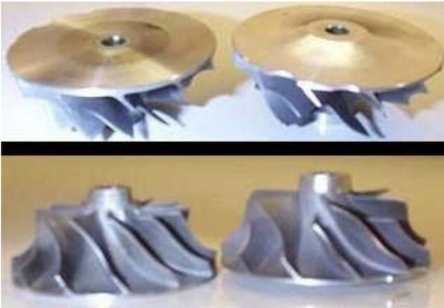
The 14B compressor wheel is on the left, the 16G on the right. Note that the back of the 14B wheel is flat, while the 16G is tapered. If you were to put a 16G wheel on a 14B center plate, the wheel would be sitting too high on the center section.
