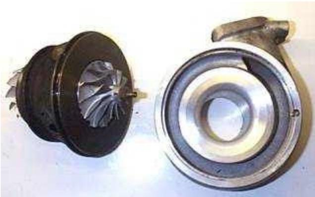
Center section removed from the compressor housing.
