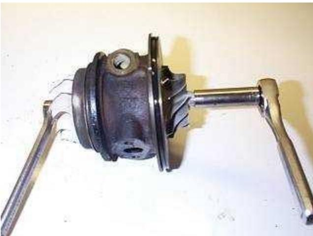
***If you are not sending your turbo for a full rebuild, MAKE SURE to scribe a line across the compressor wheel, nut, and the end of the shaft at this time. If you do not bolt it back together with ALL of the lines lined up, your turbo may end up being out of balance, and it can quickly destroy itself.***
