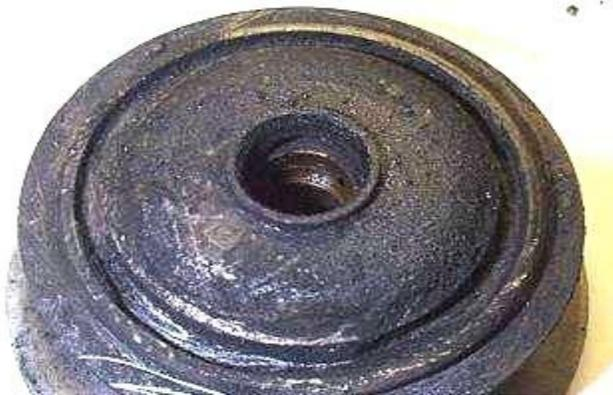
This is after about 5 minutes of chipping the coking away by tapping it with a flat blade screwdriver, sometimes tapping very hard. It still needed further cleanup, soaking it for several hours in solvent should have done it, but I had Forced Performance bead blast it while they were doing other work to it.
