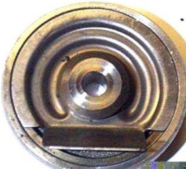
The center cap with the spring-loaded plate on it. This pushes the thrust bearing against the turbine shaft, to keep it from moving end-to-end.
