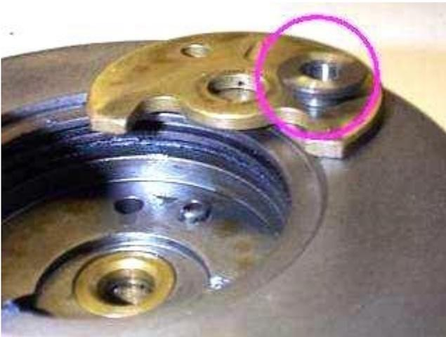
The steel bushing out of the thrust bearing. *Note that the thrust bearing and its' steel bushing are upside-down in this picture.*
