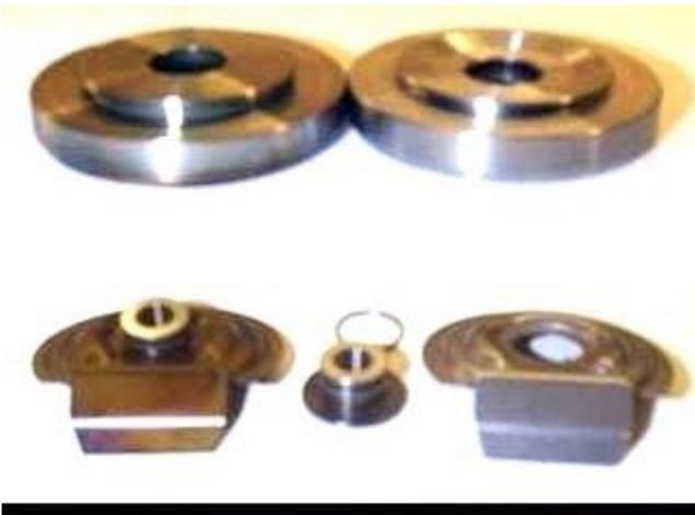
The 14B center plate is on the left, the 16G on the right. Note the taper on the 16G plate.
