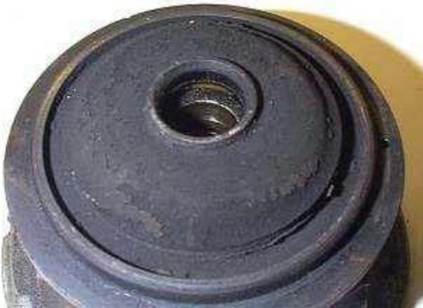
*Good* center section - still a little coking, but minimal, and easily cleaned up.
