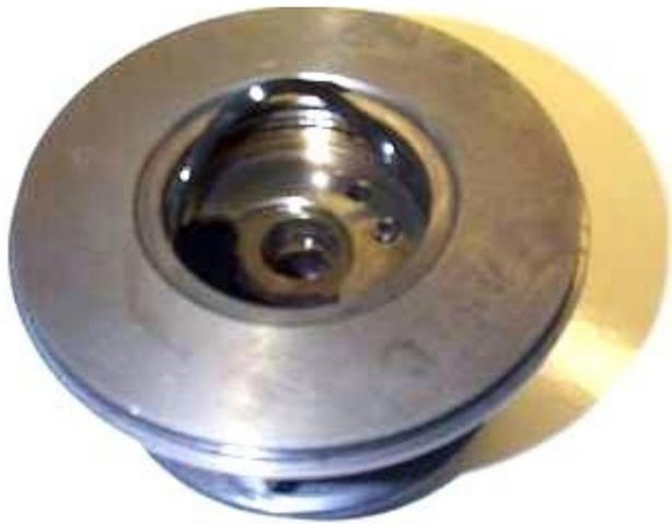
Remove the end cap O-ring. Here the O-ring is part way out. Then clean the entire center section thoroughly. Brake parts cleaner works well.
