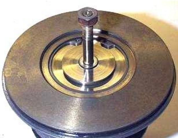
Put the nut back on the shaft, spin it on flush with the end of the shaft, and tap it *lightly* with a hammer to knock the turbine wheel/shaft assembly out of the center section.
