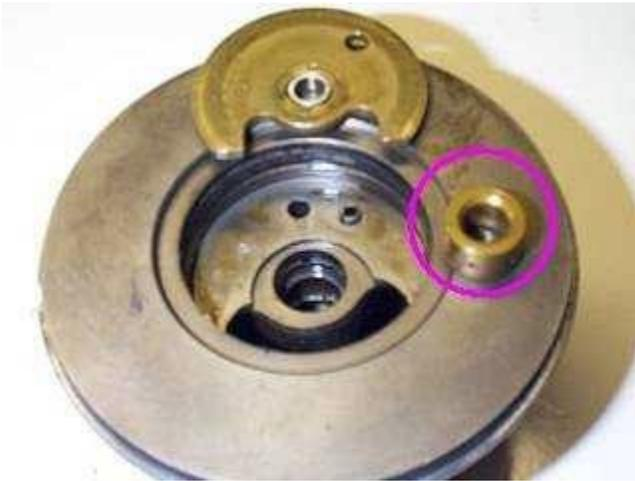
The compressor side turbine shaft bushing removed from the center section.
