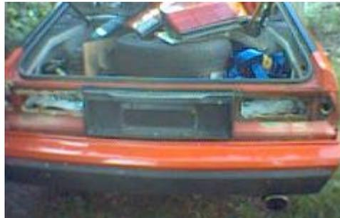
This picture shows the Rear lights removed, with the old garnish on.
