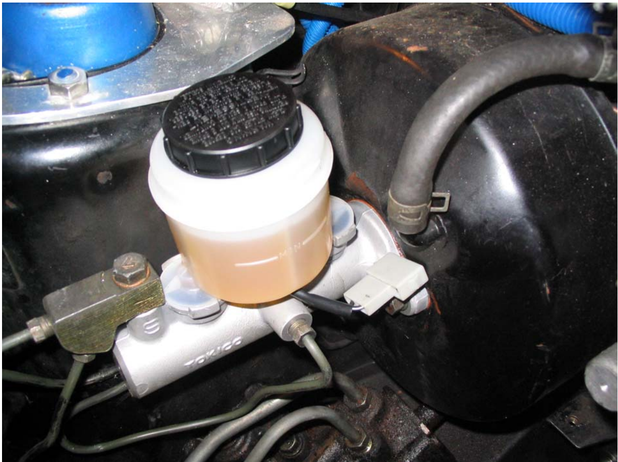
FIG 9: TOKICO 17/16 INCH MASTER CYLINDER ON JA STARION BRAKE BOOSTER
